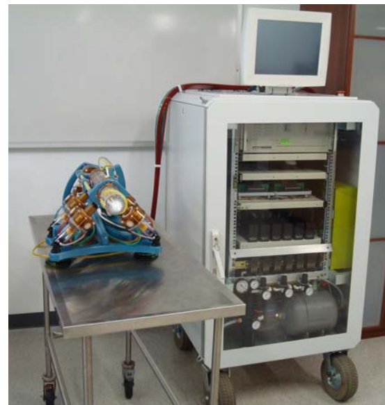
Fig. 3. MR compatible robot developed for prostate brachytherapy.
