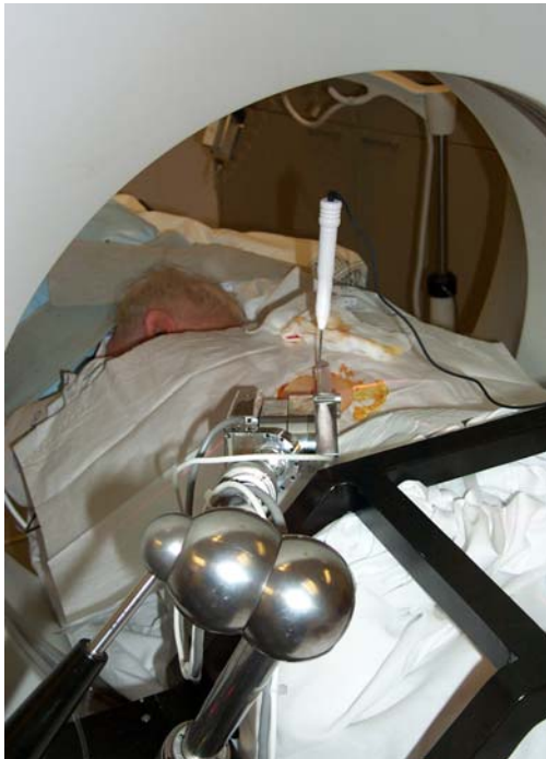
Fig. 2. IGI RF kidney ablation using the PAKY-RCM robot in CT scanner.
